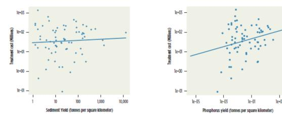
Figure 4.23. Relationship between sediment/nutrient loads and water treatment costs (TNC and IWA 2014)
