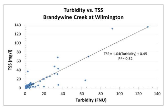
Figure 4.10. Turbidity and sediment USGS stream gage and DNREC water quality monitoring station at Brandywine Creek at Wilmington
