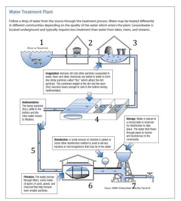
Figure 4.20. Water Treatment Plant Process (USEPA 2009)
